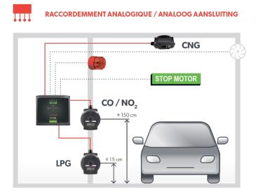
The U•V6 unit also has internal fault management. Notification is sent via a relay signalling a technical fault once any unusual use of the unit or a detector is detected. This function thus ensures the reliability of the gas-detection system installed.
