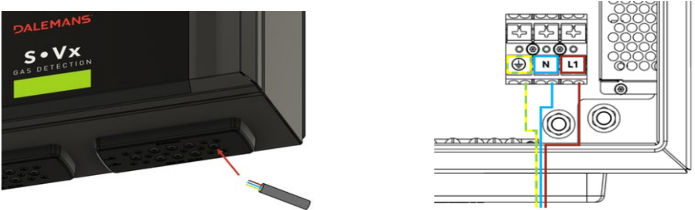
Figure 27 – Cable entry (left) and schematic wiring diagram of power supply (right)
